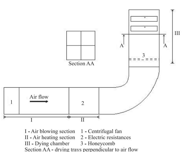
**Figure 1.** Schematic diagram of resistive dryer with crossed airflow.
