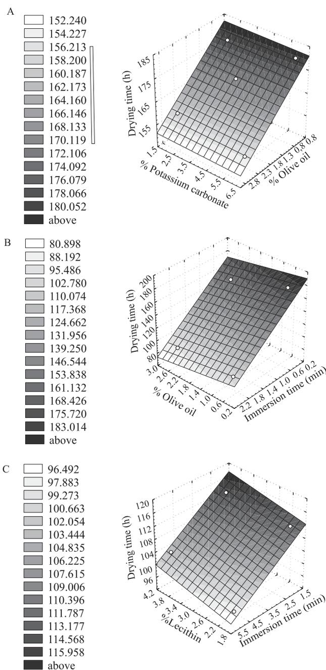
**Figure 3.** Effect of pretreatment conditions on drying time necessary to produce grapes with final moisture content of 14% (wet basis). (A) Different olive oil and  $K_2CO_3$  concentrations with immersion time of 30 seconds. at 50°C. (B) Different olive oil concentrations and immersion times in a 6%  $K_2CO_3$  solution at 50°C. (C) Different lecithin concentrations and immersion times at 50°C.
